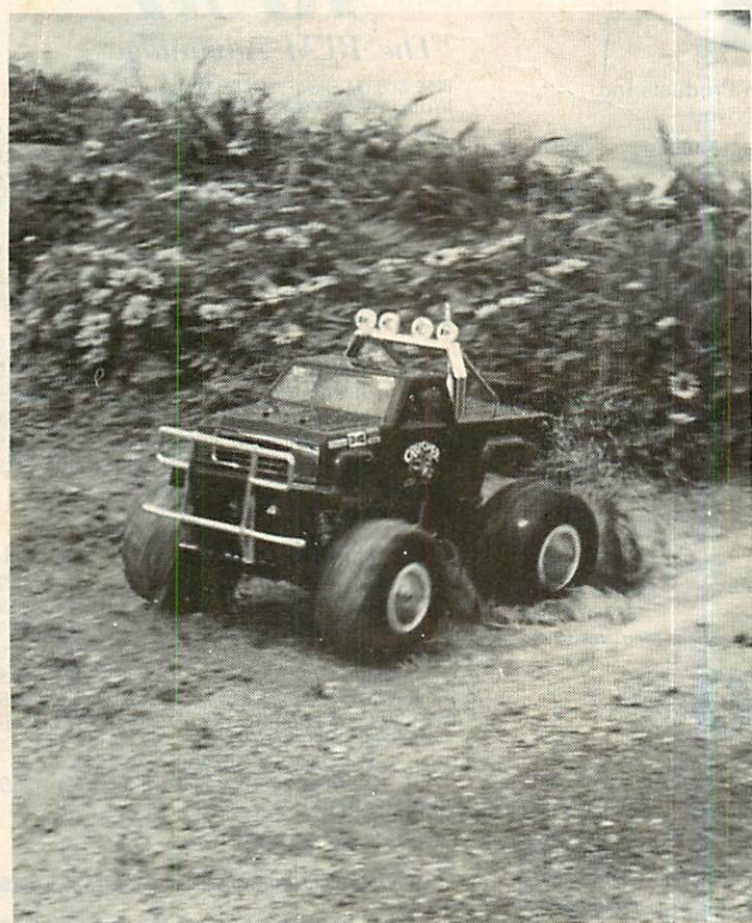
Motor is outboard at the rear and needs to be protected from the mud and dirt by a filter.
