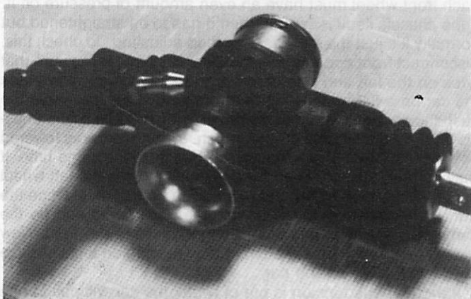
The carburettor casing is plastic, which is both light and durable, but all the internals are metal.
