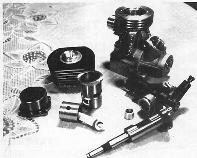
The component parts. Note polished end plate, chrome plated brass liner and well finished crank.
